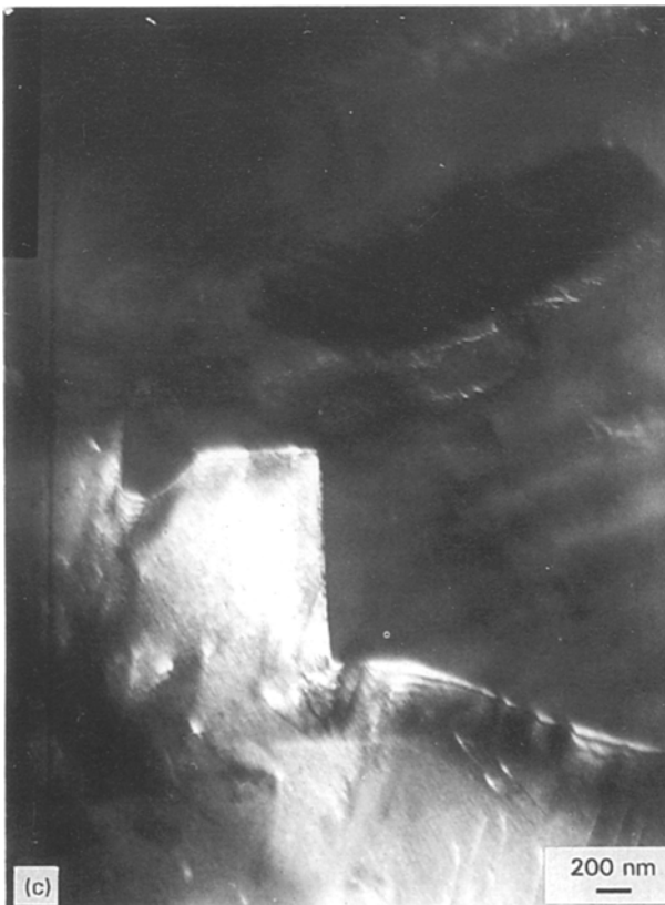
Figure 5 TEM micrographs of microstructures of ribbon N2. (a) Bright field; (b) SAED pattern of Y' , [01\bar{1}] zone; (c) dark field of Y' in (a).
