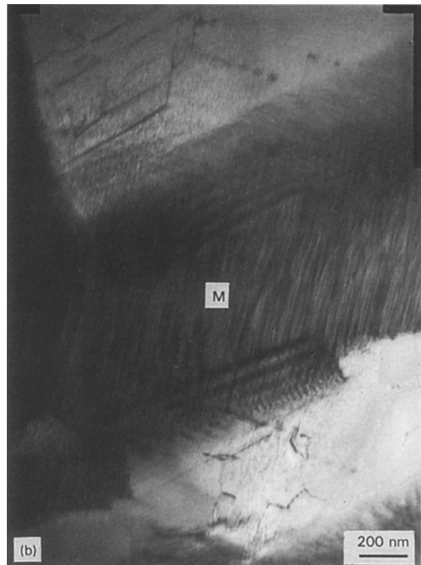
Figure 6 TEM micrograph of dislocations in ribbon N2. (a) Dislocations with high density in \gamma' ; (b) dislocations in \beta ; (c) inclined dislocations in the side of \beta on the interface between \beta and \gamma' .
