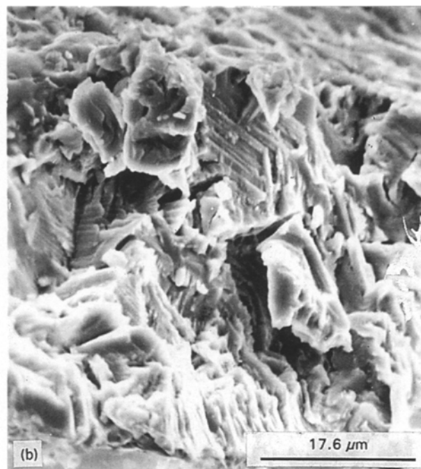
Figure 10 SEM micrographs of bent fracture surface; (a) Ribbon N2; (b) ribbon N3; (c) ribbon N4.
